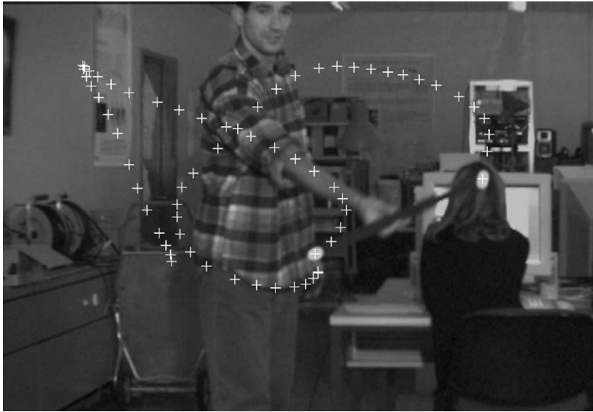
Fig. 1. Automatically tracked and measured image coordinates of the two points on the reference bar.
