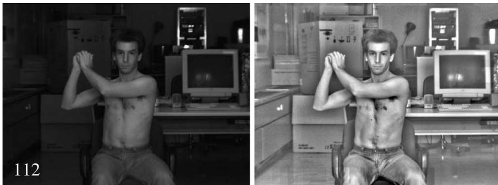
Fig. 17. A frame of an acquired sequence (courtesy of the Computer Graphics Lab, EPF Lausanne). Left: original image, right: after Wallis filter contrast enhancement.
