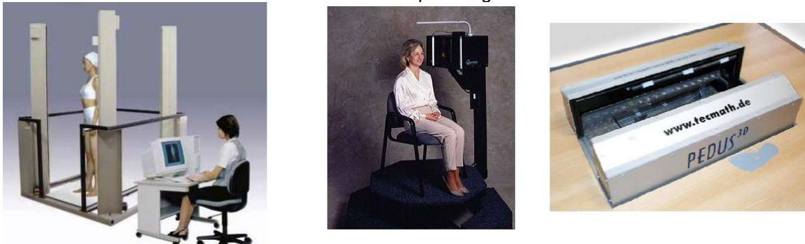
Figure 2: Laser scanning systems. Left: full body scanner BodyLine of Hamamatsu (Japan). Center: head scanner Head & Face 3030 3D Color Scanner of Cyberware (USA). Right: foot scanner Pedus of Vitronic (Germany).
