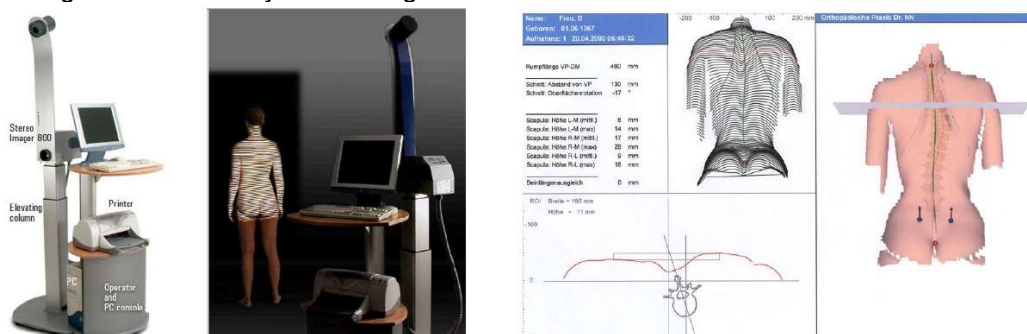
Figure 11: Human back measurement system Formetric 3D/4D [3] (Germany). Complete system (left), system in use (center), application software (right).
