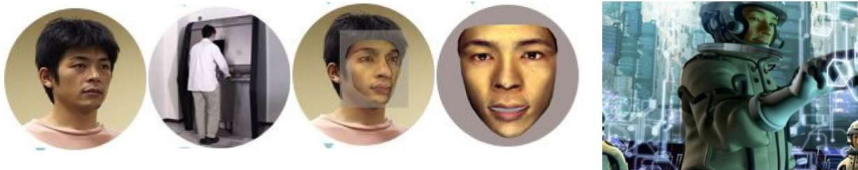
Figure 14: Futurecast system (Japan). Left: Spectator original face, face scanner, 3D face model and parametrized face mask. Right: person's face inserted and animated in real-time in the movie.
