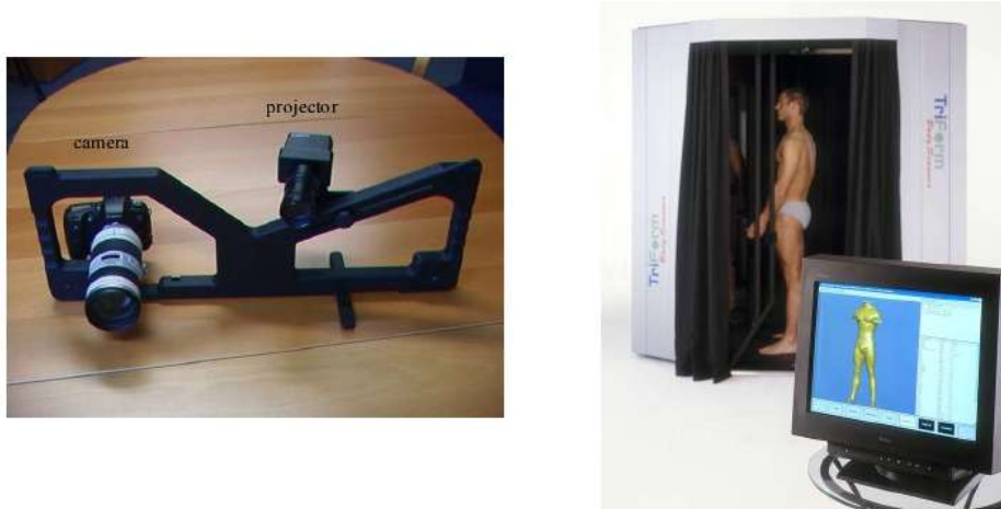
Fig. 4. Left: scanning systems with projection of light: Shapesnatcher of Eyetronics (camera and projector). Right: full body scanner TriForm of Wicks and Wilson.
