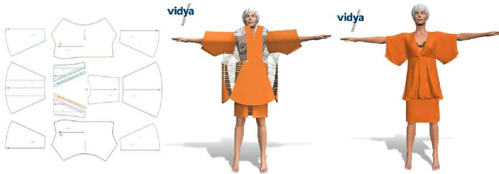
Fig. 15. Example of virtual-try-on solution Vidya of Assyst-Bullmer GmbH (Germany). Left: 2D patterns of the different parts composing a cloth item. Center: the different parts are placed in a 3D environment around the digital human body model and are stitched together. Right: the final result of the simulation.
