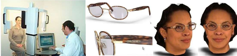
Fig. 18. Example of 3D virtual-make-over. Left: 3D acquisition system 3D iView of Visionix Ltd. (Israel). Center: 3D model of frame and lenses. Right: virtually placed eyewear onto a 3D face model.
