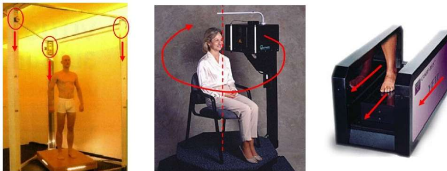
Fig. 5. Laser scanning systems. Left: full body scanner Vitus LC of Vitronic GmbH (Germany). Center: head scanner HS 3030RGB/PS of Cyberware Inc. (USA). Right: foot scanner Yeti of Vorum Research Corp. (Canada).
