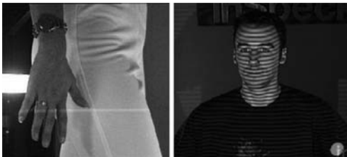
Figure 31.1. Left: laser stripe projected onto the human body. Right: structured light in the form of multiple white stripes projected onto the human body. (see colour plate page 515)
