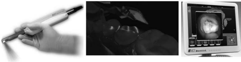
Figure 31.14. The intra-oral scanner E4D Dentist of D4D Technologies (2008): the hand held miniaturized scanner (left), surface scanning by multiple lines projection (centre), real-time scanning control visualization (right). (see colour plate page 518)
