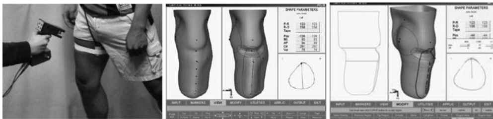
Figure 31.11. Lower limb socket design system CANFIT PLUS P&O: hand-held laser scanner and snapshots of the CAD/CAM solution. (see colour plate page 517)
