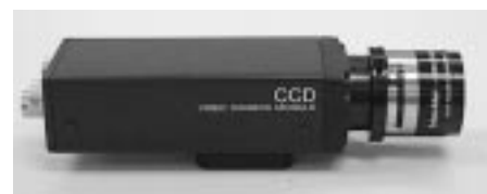
Fig. 2: CCD camera with 35 mm lens
