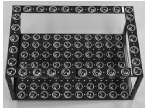
Fig. 6: 3-D calibration frame with coded targets
