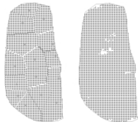
Fig. 8 Regularization and filtering results. Left: template matched points and seed points. Right: after regularization and filtering.
