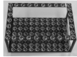
Fig. 2 Calibration frame with coded targets.
