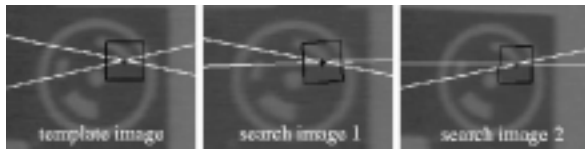
Figure 5. Geometrical constrained LSM; left: template image, center and right: two search images
