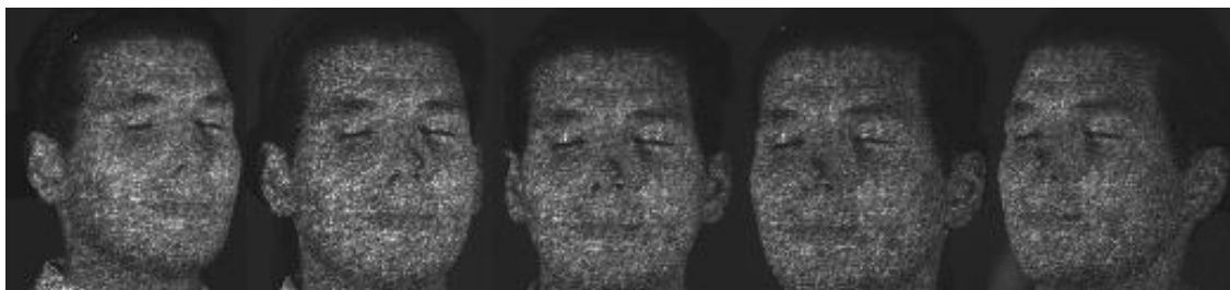
Figure 3. Multi-images of a face with random pattern projection
