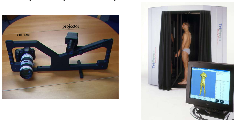
Fig. 4. Left: scanning systems with projection of light: Shapenatcher of Eyetronics (camera and projector). Right: full body scanner TriForm of Wicks and Wilson.
