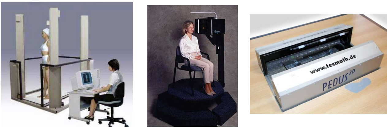
Fig. 2. Laser scanning systems. Left: full body scanner BodyLine of Hamamatsu. Center: head scanner Head & Face 3030 3D Color Scanner of Cyberware. Right: foot scanner Pedus of Vitronic.
