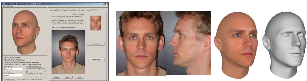
Fig. 6. Face modeler Facegen . Left: snapshot of software. Center: used images for the generation of the virtual head. Right: generated 3D face model with and without texture (images of Singular Inversions).
