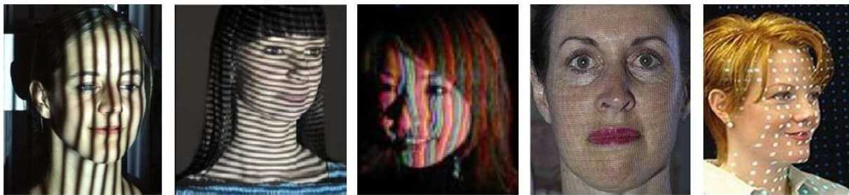
Fig. 7. Examples of projected light pattern. From left to right: vertical stripes by 3D-Shape GmbH (Germany), horizontal lines by Wicks and Wilson Ltd. (UK), color coding by Sanyo Electric Co.Ltd. (Japan), squared pattern by Eyetronics NV (Belgium), dot pattern by VX Technologies Inc. (Canada).
