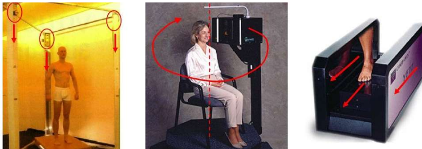
Fig. 5. Laser scanning systems. Left: full body scanner Vitus LC of Vitronic GmbH (Germany). Center: head scanner HS 3030RGB/PS of Cyberware Inc. (USA). Right: foot scanner Yeti of Vorum Research Corp. (Canada).
