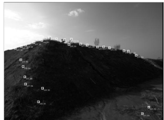
Figure 13. Tracking Result using HARRIS operator and SSDA Template Matching
