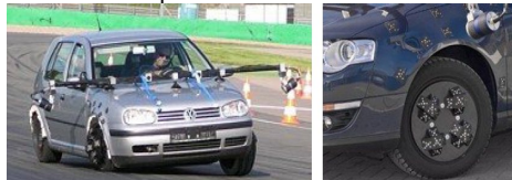
Figure 27: Wheel-Watch system during test driving (left), coded marks on the car body and on the wheel (right).
