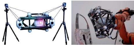
Figure 26: Combined system naviSCAN3D . Left: setup, stereoSCAN3D with reference cage and photogrammetric measurement system. Right: naviSCAN3D mounted on a robot.
