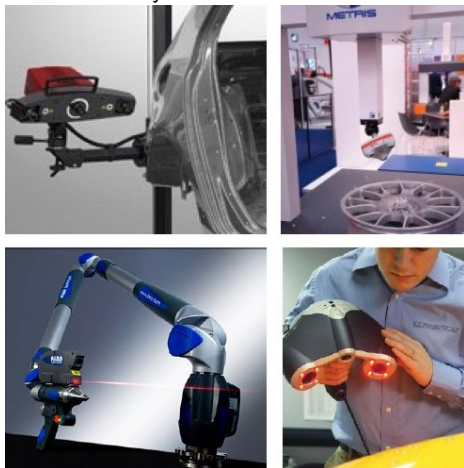
Figure 25: Left up to bottom right: fringe projection system ATOS by GOM mbH, laser profiler XC50-LS mounted on CMM by Metris, hand-operated laser profiler on mechanical arm Laser Scan Arm V3 by FARO, hand-held scanner EXAscanner by Creaform.
